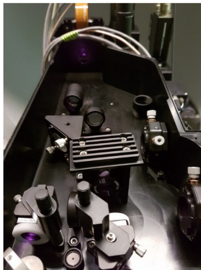
Figure 4: Stimulation light path with spatial modulator which the BlueCut laser is integrated into.
